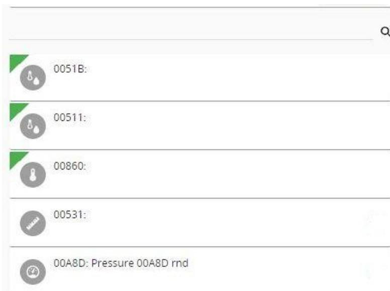
Each time new sensor is successfully paired, 2-minutes timer is restarted. If sensor pairing was not successful within 30-seconds period, take out battery from the sensor, wait 10 seconds and place battery back to repeat pairing process. When you finish pairing all sensors, press "STOP PAIRING" button or wait for the timer to close pairing process automatically.
