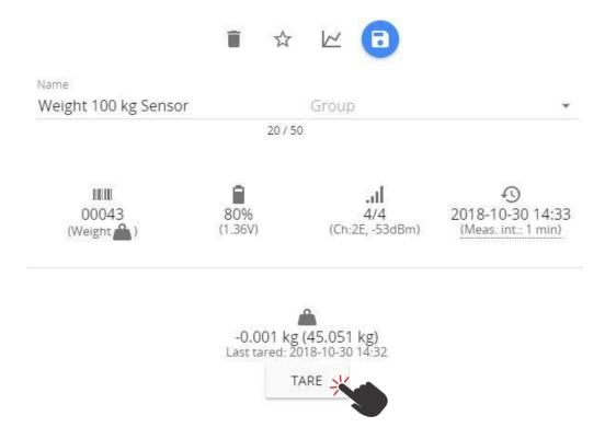
By default, the graph of the **Weight Sensor** will display measurements of a tared weight. To display the untarred weight in the graph, click the **Tune** tick the **"Show"** box.
