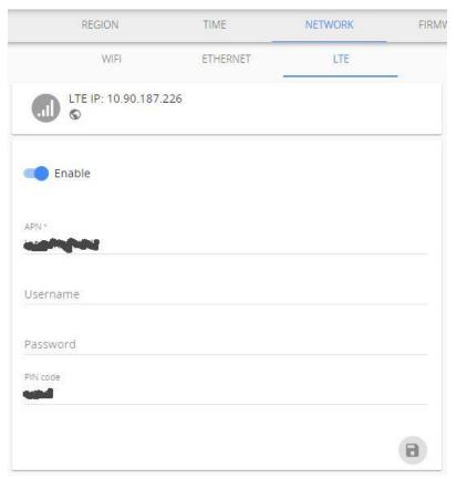
It is possible to access the Aranet PRO Plus LTE web interface from the Internet over an LTE connection. For this purpose, please contact your Mobile Internet provider and request the static IP-address for the SIM-card inserted into modem.
