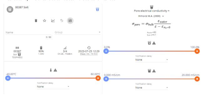
Use the **Tune** button (in the Graph section), to display the Bulk Electrical Conductivity and dielectric permittivity ( $\epsilon$ ).
