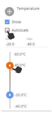
To display the measurement curves with more granularity, untick the **Autoscale** and choose the Min and Max values by moving the slide bars or typing in the required values.
