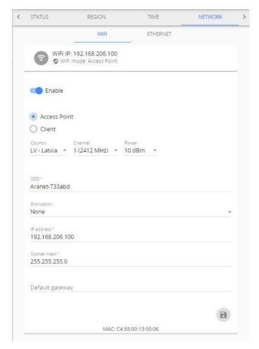
(2) In case you wish to connect an Aranet PRO/PRO Plus to a local Wi-Fi network, choose the **Client** mode, find the appropriate Wi-Fi connection, and fill in the Wi-Fi password. Apply the changes by using the **Save** button.
