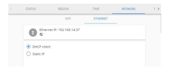
In case of static IP, select **Static IP** and fill in all needed fields: *IP address, Subnet Mask, Default gateway* and *DNS server*, an **example** is shown in the picture below, and click **Save**. Consult your network administrator for these parameters in your local network.
