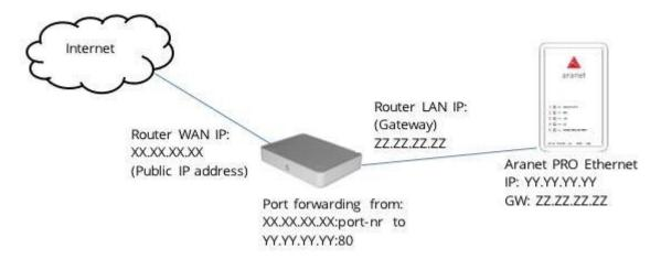
For accessing Aranet PRO/PRO Plus, open the Internet browser and in the URL bar, type the IP address with port number, xx.xx.xx:port-nr (for instance, 213.100.100.1:8100).
