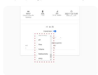
**9.** To do that switch the Conversion on, and use the drop-down menu to choose a predefined Dimension and unit.
