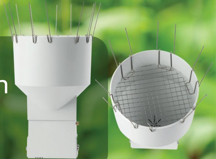
Aranet Rain and Precipitation sensor kit is specifically designed for outdoor monitoring of rain and precipitation. This versatile kit finds applications in agriculture for irrigation and soil moisture management, weather stations, water treatment plants, and more.
